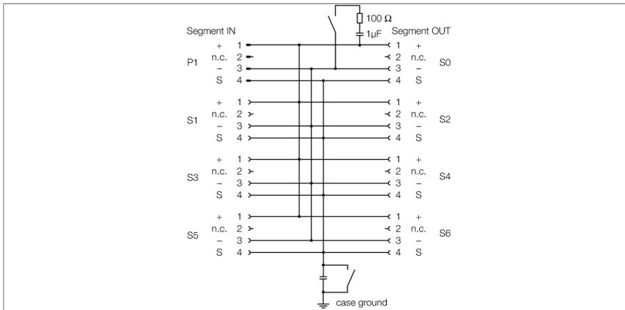
The 6-channel Ex junction box JBBS-48-E613/EX is designed for PROFIBUS-PA systems.
