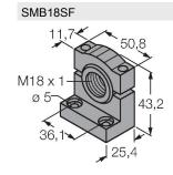
Mounting bracket, PBT black, for sensors with 18 mm thread, rotatable
