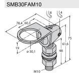
3011185 Mounting bracket, stainless steel, for M10 x 1.5 thread, thread length 30 mm
