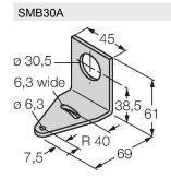
Mounting bracket, rectangular, stainless steel, for sensors with 30mm
