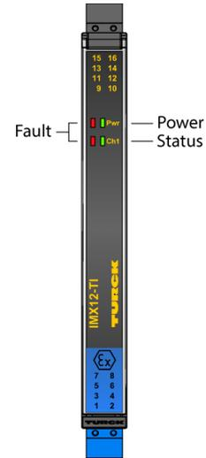
The temperature transducers in the IMX12-TI02... product series are equipped with intrinsically safe input circuits and can be used for the galvanically isolated transmission of temperature-dependent measured values from the Ex area to the non-Ex area. The devices are suitable for operation in Zone 2. Thermocouples, low voltages, RTD sensors and resistors can be connected to the devices in the Ex area.
