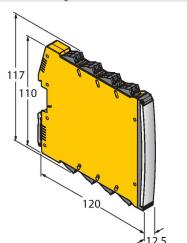
Isolating switching amplifier, 2-channel; SIL2 acc. to IEC 61508; Ex-proof version; 2 transistor outputs; input Namur signal; ON/OFF switchable monitoring of wire-break and short-circuit; toggle between NO/NC mode; signal doubling; removable screw terminals; 12.5 mm wide; 24 VDC power supply
