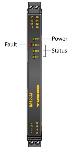
The IM12-AI01-1I-1IU1R-H... isolating transducers transmit the analog measured signal in a galvanically isolated manner. In addition, the devices monitor the input signals for exceeding or falling below an adjustable limit value. The devices are suitable for operation in Zone 2. Passive 2-wire transducers, as well as active and passive HART transmitters, can be used on the devices.
