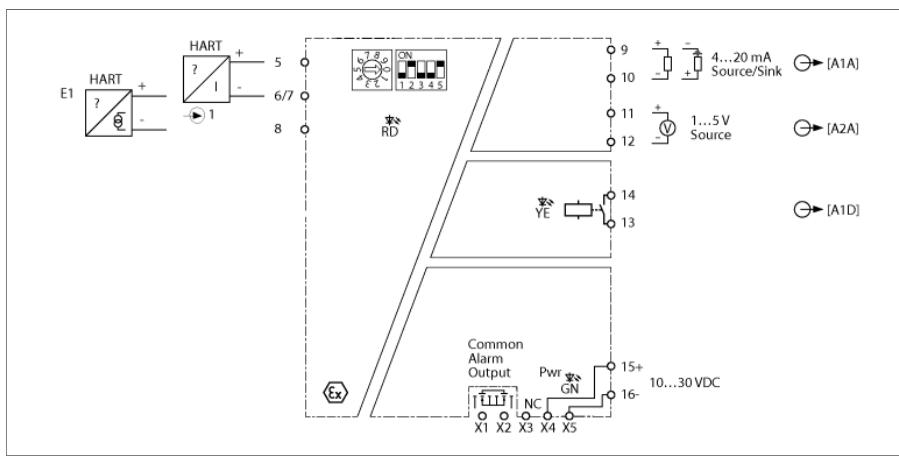
The IMX12-AI01-1I-1IU1R-H... isolating transducers are equipped with intrinsically safe input circuits and transfer analog measured signals from the Ex area to the non-Ex area. In addition, the devices monitor the input signals for exceeding or falling below an adjustable limit value. The devices are suitable for operation in Zone 2. Intrinsically safe (passive) 2-wire transducers, as well as active and passive HART transmitters, can be used on the devices in Ex areas.
