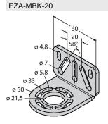
Mounting bracket, steel, blackfinished, for EZ-ARRAY and EZ-SCREEN standard 14 & 30 mm
