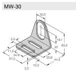
6945005 Mounting bracket for threaded barrel sensors; material: Stainless steel A2 1.4301 (AISI 304)
