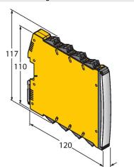
Isolating switching amplifier, 2-channel; SIL2 acc. to IEC 61508; Ex-proof version; 2 transistor outputs; input Namur signal; ON/OFF switchable monitoring of wire-break and short-circuit; toggle between NO/NC mode; signal doubling; removable screw terminals; 12.5 mm wide; 24 VDC power supply
