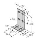
Mounting bracket, for PVA and PVD, stainless steel; set consisting of two brackets and screws
