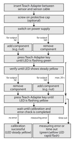
The measured signal in the sensor is influenced by the diameter and the material characteristics of the center bolt, but also by the cover of the sensitive area. Therefore each sensor has to be conditioned to the operating environment, i.e. to the applied sleeves or closure caps and the target (nut, sleeve etc.) To configure a sensor, the teach adaptor VB2-SP1 available from Turck is required.
