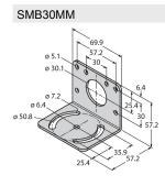
3027162 Mounting bracket, rectangular, stainless steel, for sensors with 30 mm thread, wide holes for accurate alignment
