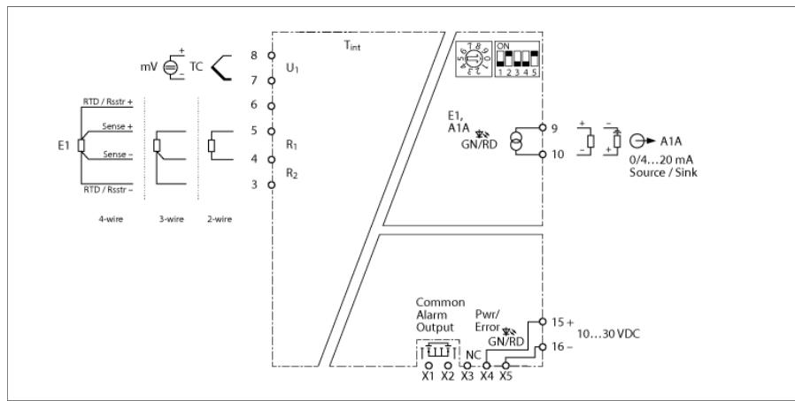
The temperature transducers of the IM12-TI02... product series transmit temperature-dependent measured values in a galvanically isolated manner. The devices are suitable for operation in Zone 2 (ATEX region). Thermocouples, low voltages, RTD sensors and resistors can be connected to the devices in the Ex area.
