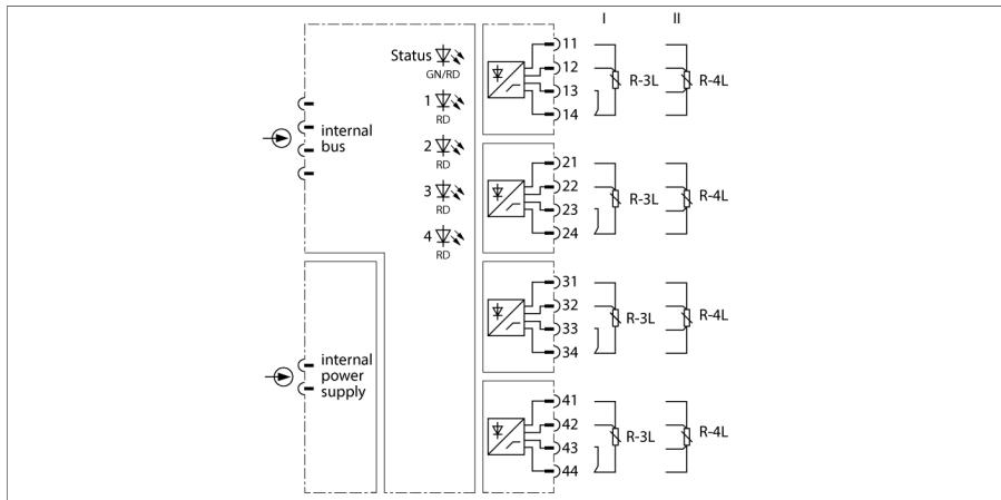
The analog input module AI43-N is used for the connection of potentiometers in 3 or 4-wire technology. If 3-wire potentiometers are used, the terminals at the module rack have to be bridged. Resistance measurements, i.e. the evaluation of potentiometers with a 2-wire connection, is not possible.
