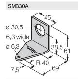
3032723 Mounting bracket, rectangular, stainless steel, for sensors with 30mm thread
