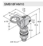
3011184 Mounting bracket, material VA 1.4401, for M10 x 1.5 thread, thread length 18 mm
