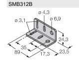
Mounting bracket, stainless steel, for MINI-BEAM NAMUR
