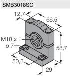
3053952 Mounting bracket, PTB black, for sensors with 18 mm thread
