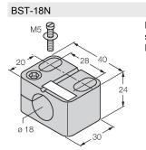
6947215 Mounting clamp for threaded barrel sensors, without dead-stop; material: PA6
