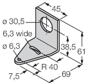
Mounting bracket, rectangular, stainless steel, for sensors with 30mm thread
