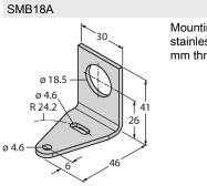
3033200 Mounting bracket, rectangular, stainless steel, for sensors with 18 mm thread
