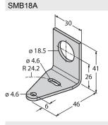
Mounting bracket, rectangular, stainless steel, for sensors with 18 mm thread
