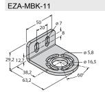
3071470 Mounting bracket, steel, blackfinished, for EZ-ARRAY and EZ-SCREEN standard and cascade 14 & 30 mm
