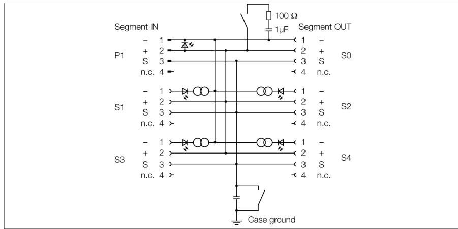
The 4-channel Ex junction box JBBS-49SC-E413/Ex is designed for FOUNDATION™ fieldbus systems.
