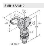
3011184 Mounting bracket, material VA 1.4401, for M10 x 1.5 thread, thread length 18 mm
