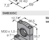
3052521 Mounting bracket, PBT black, for sensors with 30 mm thread, rotatable
