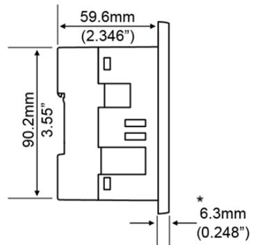
\* Note that for models V130/V350, the bezel width is up to 8.4 mm (0.33").
