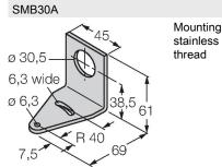
Mounting bracket, rectangular, stainless steel, for sensors with 30mm thread
