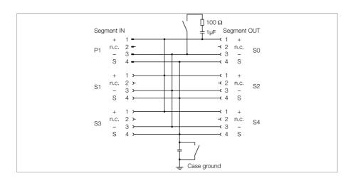
The 4-channel junction box JBBS-48-M413/3G is designed for PROFIBUS-PA systems.
