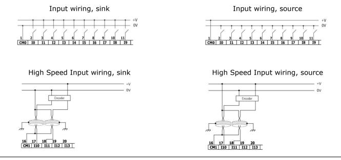
**Note** Use sink input wiring to connect a sourcing (pnp) device. Use source input wiring to connect a sinking (npn) device.
