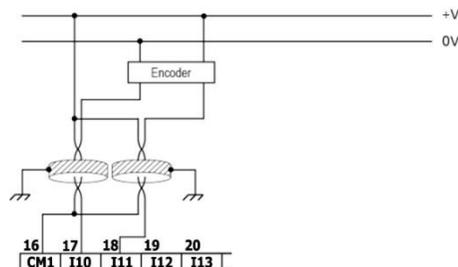
**NOTE** Use sink input wiring to connect a sourcing (pnp) device.
