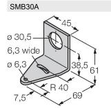
3032723 Mounting bracket, rectangular, stainless steel, for sensors with 30mm thread
