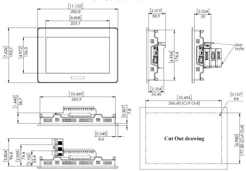
**Note** Allow space for modules to be snapped onto the back of the controller, if required by your application. Modules are available by separate order.
