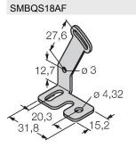
3067467 Mounting bracket, stainless steel, for 18 mm thread
