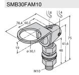
3011185 Mounting bracket, stainless steel, for M10 x 1.5 thread, thread length 30 mm
