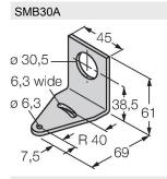
3032723 Mounting bracket, rectangular, stainless steel, for sensors with 30mm thread
