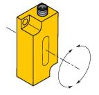
Adjusting the measuring range via TX1-Q20L60 teach adaptor
