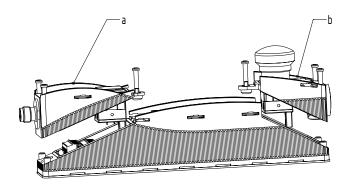
When closing the enclosure cover, ensure that the emergency stop module is flush with the bottom section and that the cover screws are screwed in as far as they will go. The emergency stop safety function must be checked by an appointed safety technician / safety representative once successfully installed.
