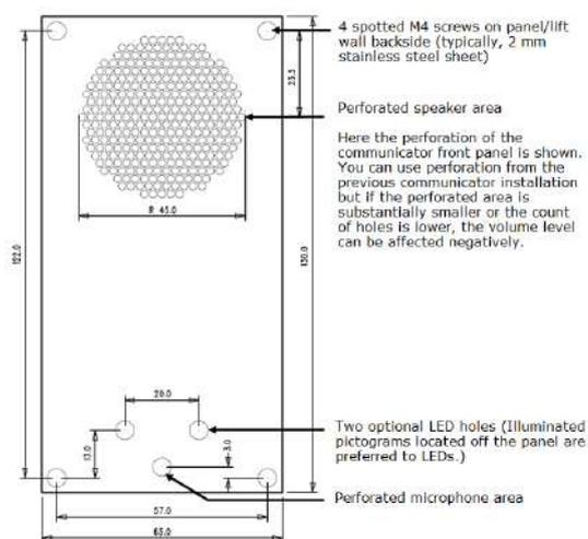
If you use other than the prescribed screws, make sure that the isolation distance between the electronics and substandard fitting elements is 2 mm at least. Make sure that the panel is fitted perfectly to avoid resonance during operation. There may be no gap between the lift button panel and the 2N® LiftIP panel, or the gap must be sealed properly to eliminate acoustic fault of the speaker and acoustic feedback between the speaker and microphone (see below).
