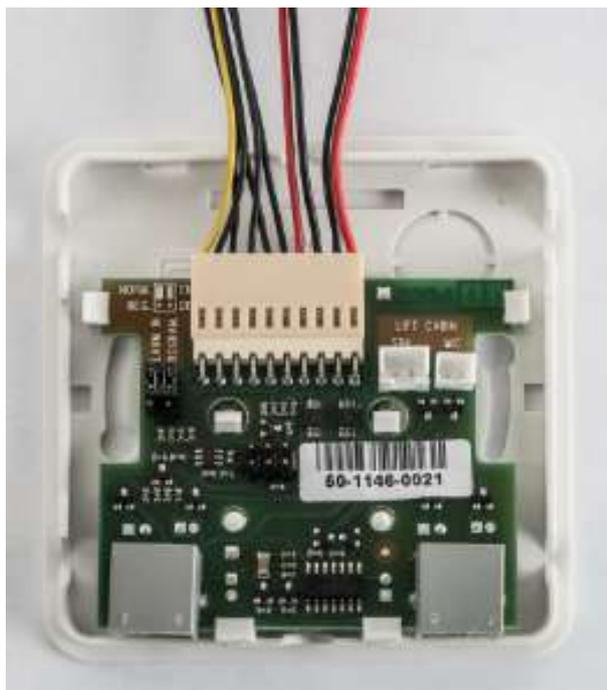
Connect the microphone and speaker from 2N<sup>®</sup> LiftIP in the switch. The speaker and microphone connectors are properly marked (SPK and MIC). Pull the cables through the holes.
