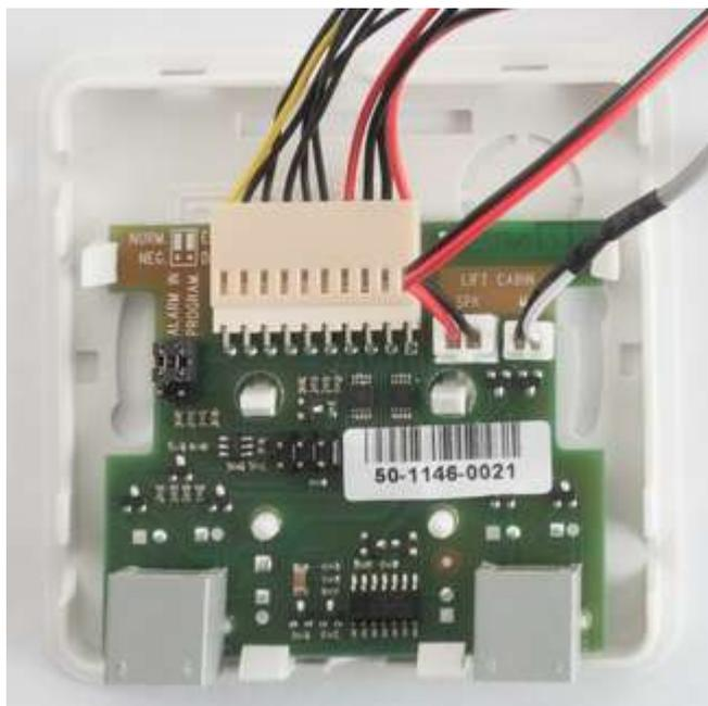
Break out the cable holes on the switch upper cover. Then replace the switch cover. Use 2 RJ-12 audio unit connectors on the switch side to interconnect the audio unit and the switch using the cable included in the audio unit package.
