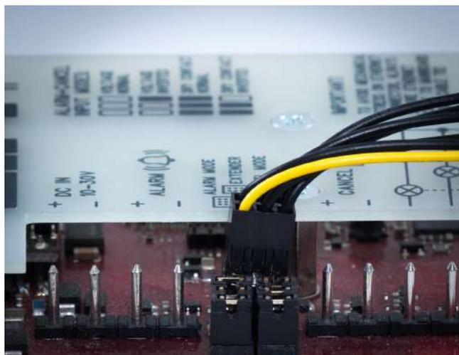
Interconnect 2N<sup>®</sup> LiftIP and the IO extender using a cable (see the figure below).
