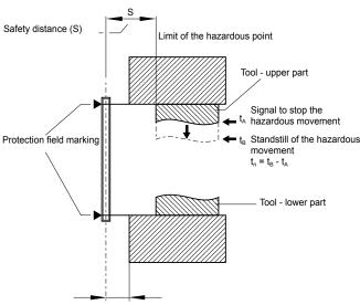
≤ 75 mm = max. distance for protection against stepping over To prevent persons from stepping over the protection field this dimension must be imperatively respected and observed.
