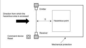
The formulae and calculation examples are related to the vertical setup (refer to drawing) of the AOPD with regard to the hazardous point. Please observe the applicable harmonised EN standards and possible applicable national regulations.
